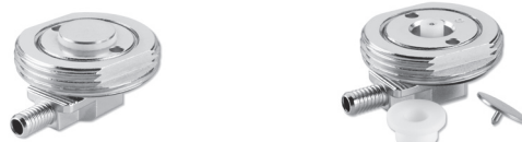
NMOHF Mount Convert from low frequency applications to high frequency applications and back by pulling or replacing the center pin and insulator.
